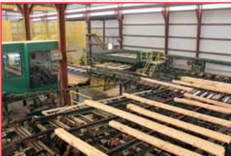
Keadle's mill processes over 50 truck-loads of logs a day. After the logs are cut, they are taken over to the kiln for drying.
