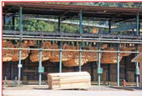
A computerized sorting system automatically shunts product to the appropriate slot. Four straps hold a pack in place. The system can output 11 or 12 packs an hour.
