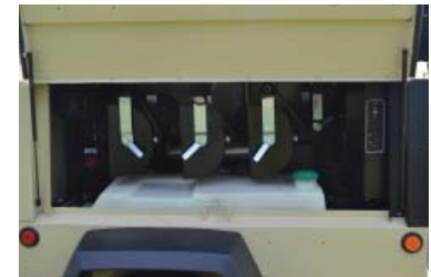
Optional internal storage for four lamp fixtures
