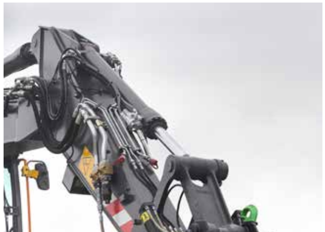
Load holding valves on bucket cylinders, both sides
