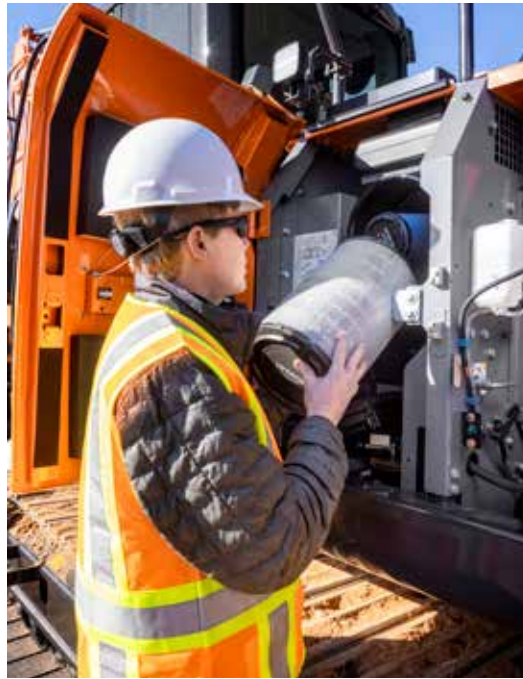
Filters within easy reach take just minutes to maintain.
