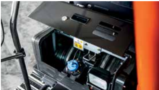
Ground-level access to urea tank
